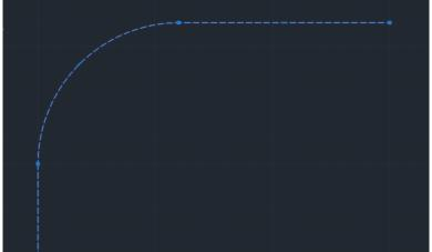
In this way we have **speeded up the design** and made the design of the Bundles that make up the harnesses more **correct and aesthetically valid**. The automatism does not occur if the angle of the line with respect to the end of the arc exceeds 15 degrees.
