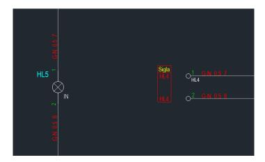
In the case of 'Insertion of graphic symbols without material', before inserting the symbols you are asked to change the values of the Pins or to confirm those already present.
